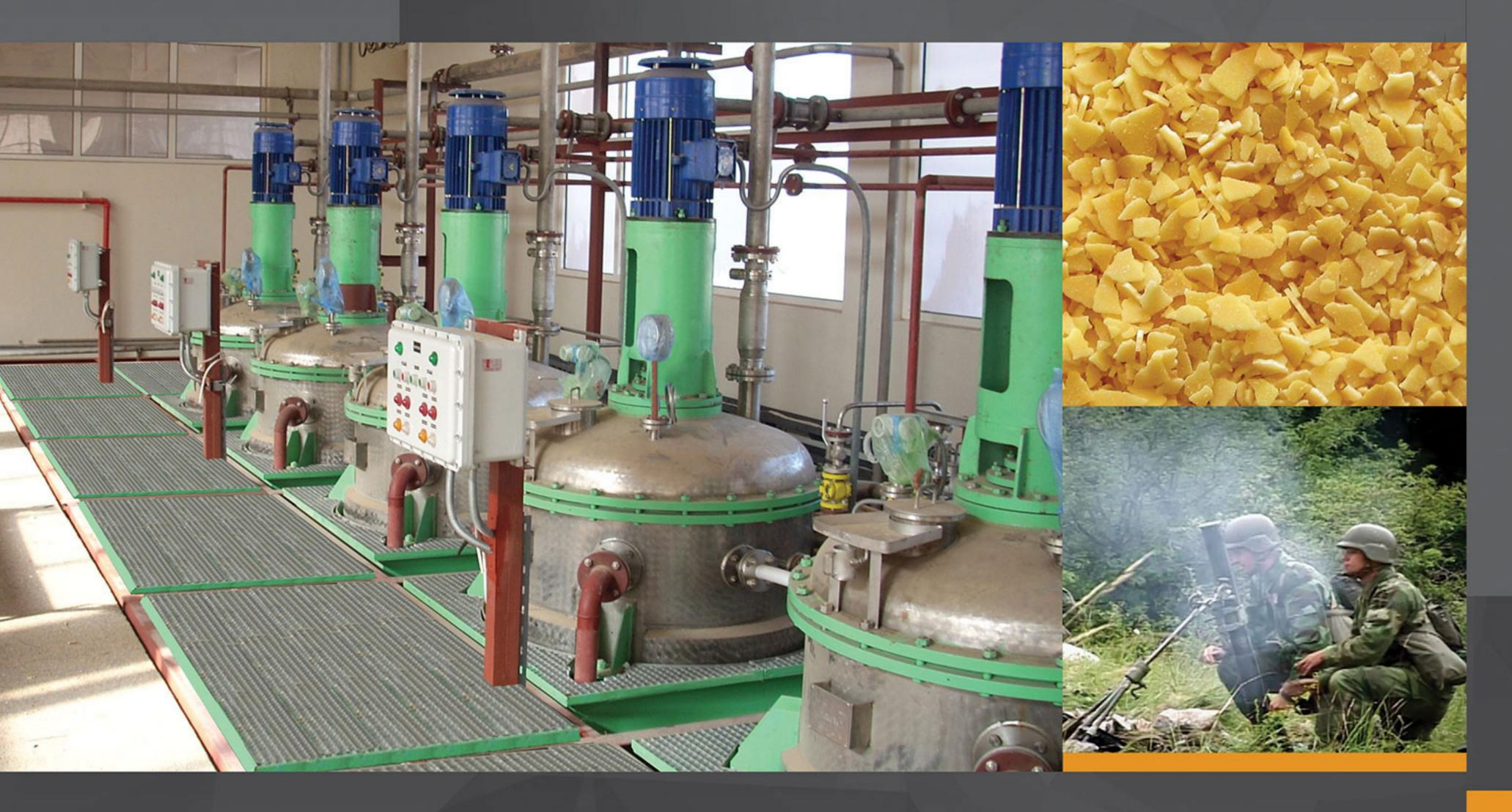
The technology is adapted for continuous production of TNT with possible using of final product for military purpose as well as for mining purpose (industrial explosive). Special emphasis has been placed on achieving a closed cycle process; this being accomplished through recovery of acids. The production process comprises a number of inter-linked manufacturing phases: synthesis (nitration), purification, drying, granulation process, packing, recovery of acids.
